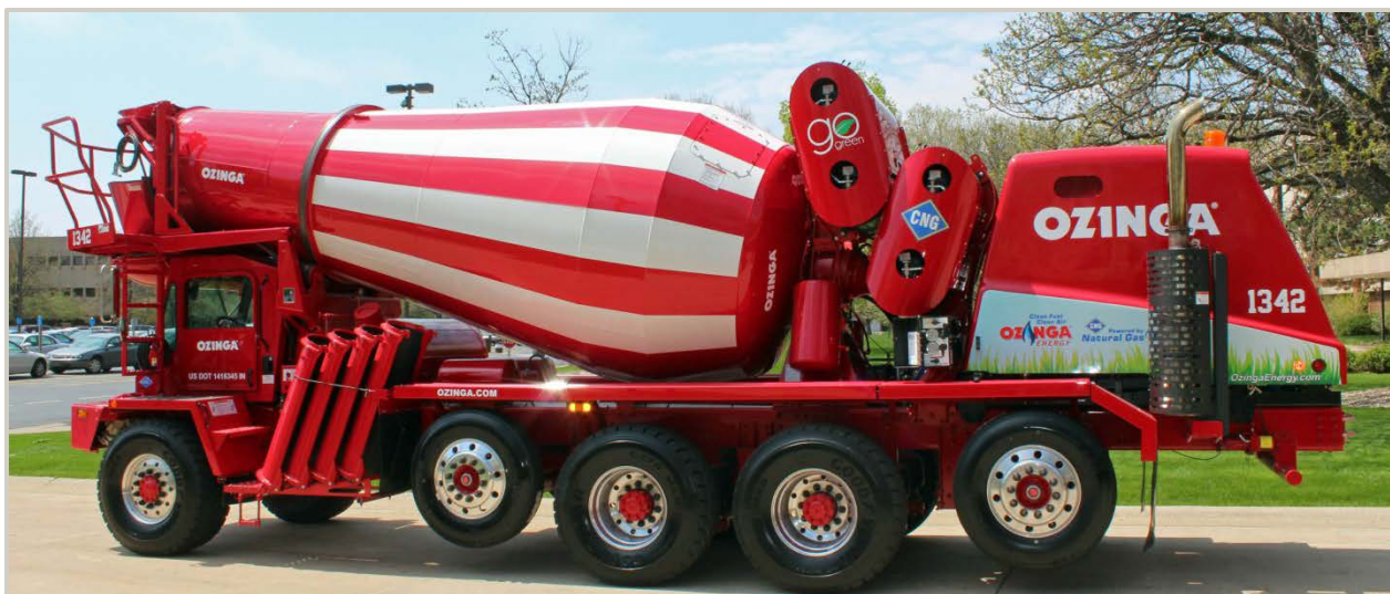
FRONT-DISCHARGE CNG CONCRETE MIXER (RETROFIT)
