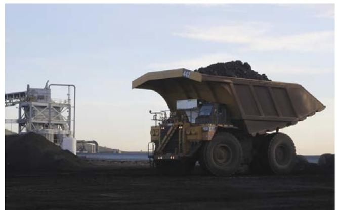
Here, one of the trucks at Alpha Coal West is shown preparing to dump a load of coal in the coal hopper. Each load is approximately 240 tons for the Cat 793. Future EVO-MT Systems are being designed for trucks with much larger capacities.
