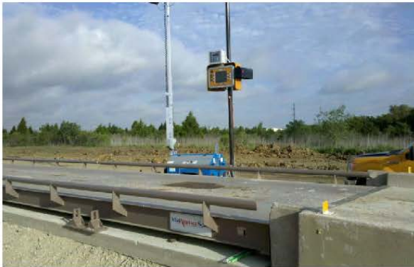
An automated scale kiosk, located on the DFW Connector project, allows haulers to record truck information electronically, eliminating manual input and error.
