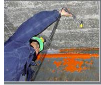
Tester apparatus and testing for strength, deterioration, and delamination
