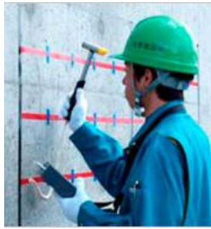
Tester apparatus and testing for strength, deterioration, and delamination
