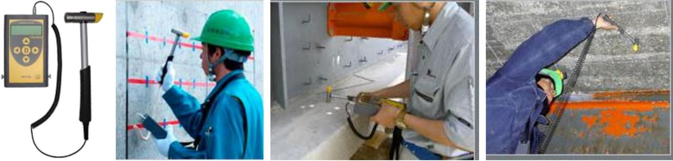
Tester apparatus and testing for strength, deterioration, and delamination
