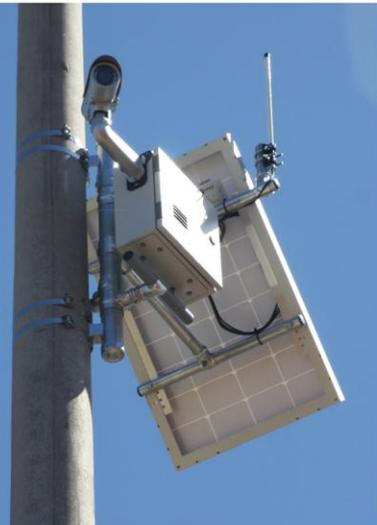
ANSO Sentinel V-Series Solar 3G Stand-alone Outdoor Web Camera System mounted at 12m on commercial shopping centre construction project.
