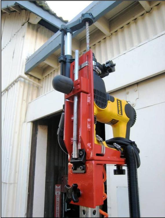
**Figure 1: Details of saddle with dust-capturing drill installed**
