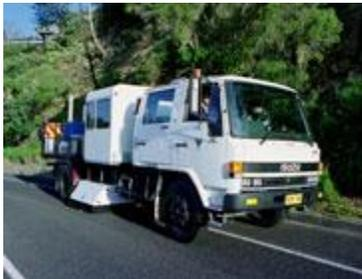
A truck fitted with RoadCrack equipment testing the road surface
