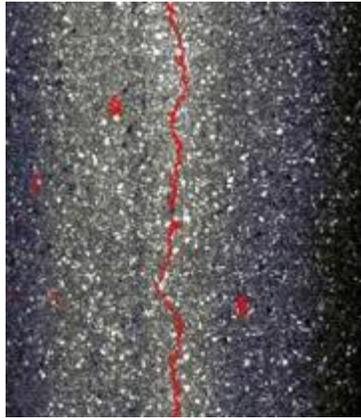
Detected crack patterns
