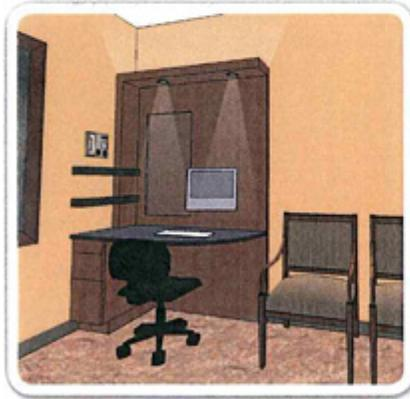
*Rapid Access Prototyping allows for hands-on, quick access approach to modifying owner requirements. Walls, fixtures, and useable space areas were created from foam core allowing for greater interaction by users and customers.*
