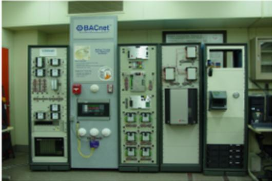
The hardware portion of the VCBT, including the HVAC controllers and data acquisition equipment.
