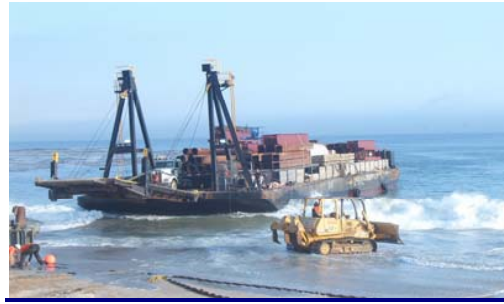
Original method of beaching barge for Offloads
