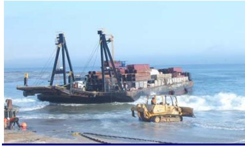
**Original method of beaching barge for Offloads**
