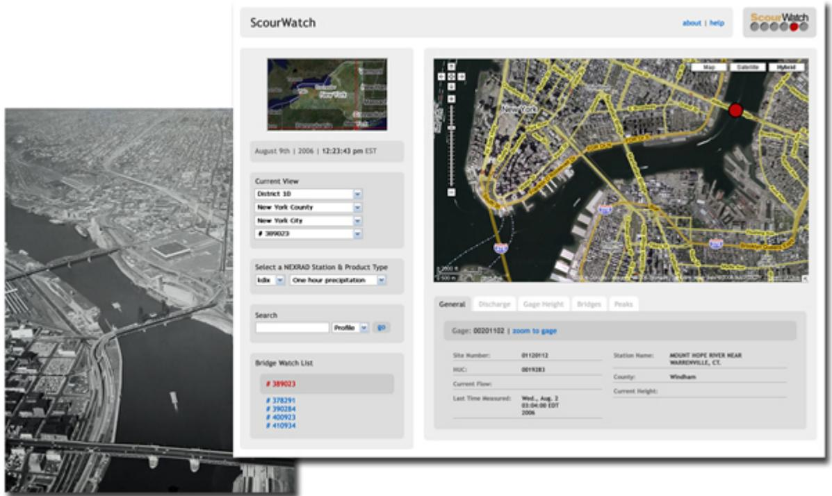
Figure 1. Scourwatch screen depicting bridge location and data.
