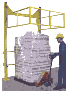
When "corral" is raised, ledge gates swing closed. Worker has access to load. Fall potential is eliminated.
