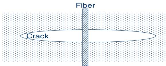
A single discontinuous conductive fiber is shown to the left. It bridges a microcrack, the opening of which is exaggerated for clarity. This is to illustrate the mechanism of the piezoresistivity in smart concrete.
