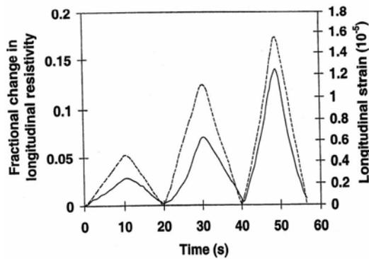
Graph to the left shows that the electrical resistivity fractional change correlates with the strain (measured with a conventional strain gage) in the same direction (longitudinal) for three loading cycles at progressively increasing strain amplitudes. Both the resistivity change and strain are reversible upon unloading.
