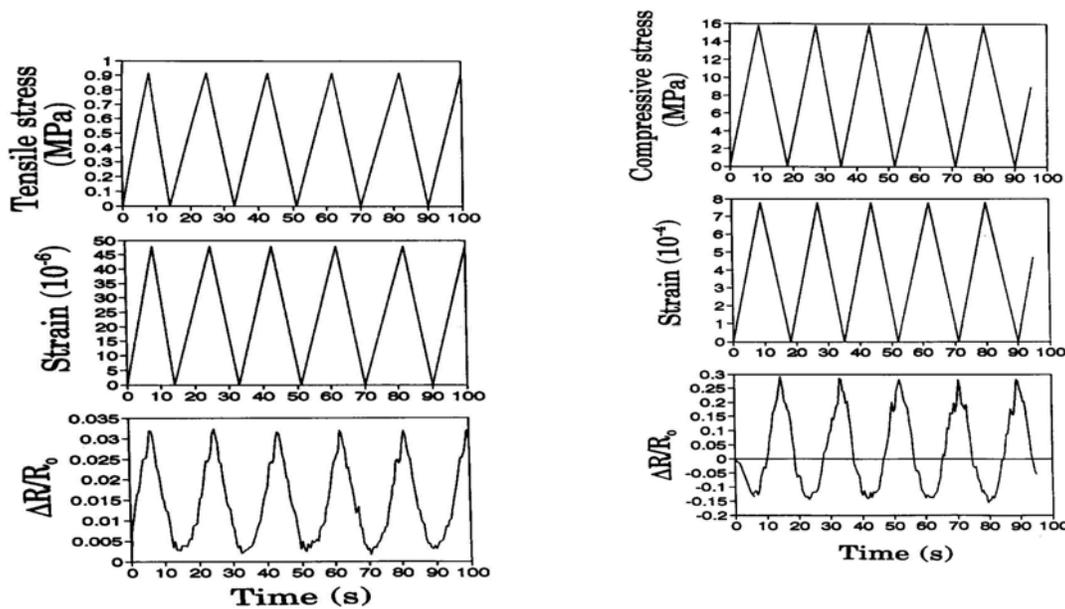
Fractional change in resistance ( $\Delta R/R_0$ ) is shown above during cyclic tension (left panel) and cyclic compression (right panel). The strain is measured with a conventional strain gage to show the correlation between strain and resistance. The resistance increases reversibly upon tensile loading and decreases reversibly upon compressive loading.
