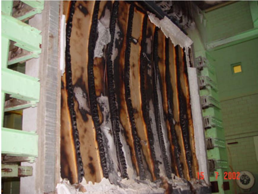
Figure 1. A Wood-Stud Wall Buckles during a Fire Test
