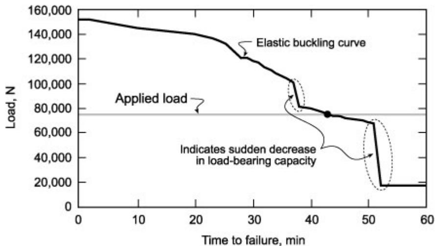
Figure 2. Typical Fire-Resistance Performance of a Wood-Stud Assembly as Predicted by Structural Response Model
