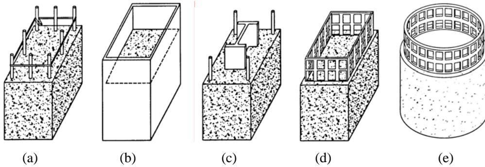
Fig. 1 a) traditional rebar reinforced (RC) system; b) concrete-filled steel tube; c) steel-concrete composite system; d and e) PCS reinforcement
