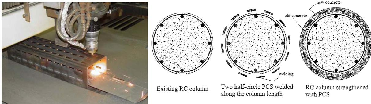
Fig. 2 PCS fabrication; and example of retrofitting deteriorated RC circular column/bridge pier using PCS
