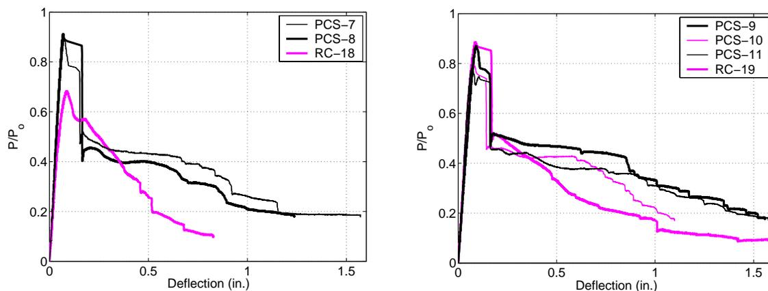
Fig. 4 Comparison of experimental normalized axial strength versus deflection relations for equivalent PCS and RC specimens shown in Fig. 3.  $P_o = A_s f_y + f'_c (A_g - A_s)$
