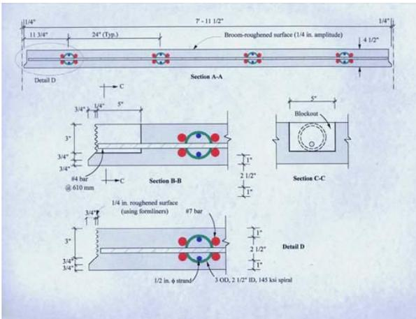
Fig.5. Details of the NUDECK SIP Panel System
