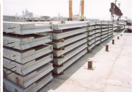
Fig. 9. Storage of NUDECK Panels in the Precast Yard
