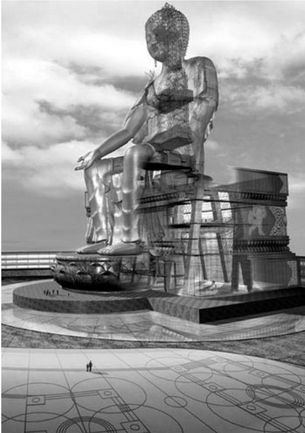
Cutaway of the 152 metre (500 ft.) Maitreya statue and throne building showing the spaces and levels within. The throne will be a 17 storey fully functional building containing 2 very large prayer halls. On the roof of the throne, stretching up into the body of the Maitreya statue, will be over 15 different shrine rooms.
