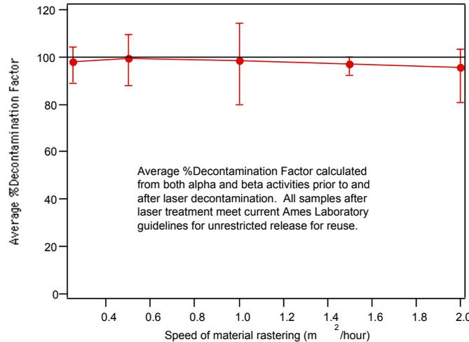
Fig. 1 Decontamination of aluminum ductwork using excimer laser
