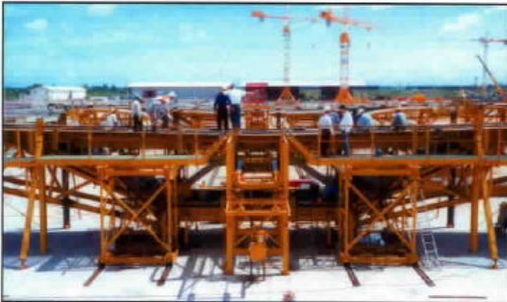
*Typical casting machine closed and ready to pour.*
