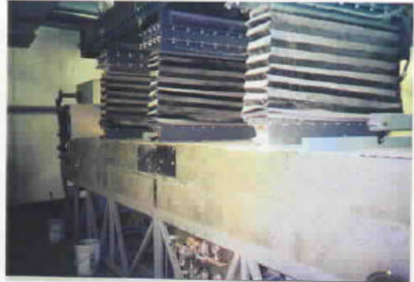
Figs. 1 and 2: Schematic drawing and photo of the state-of-the-art tribo-electric processor for removing carbon from fly ash to produce ProAsh.
