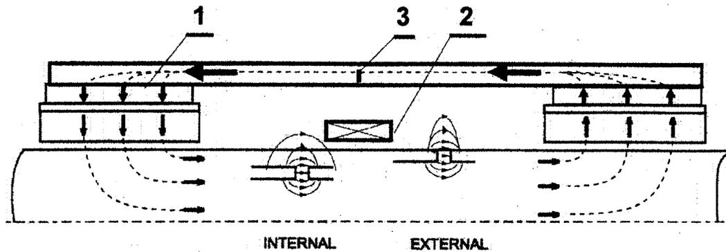
Figure 1. The principle of magnetic flux leakage inspection of wire rope
