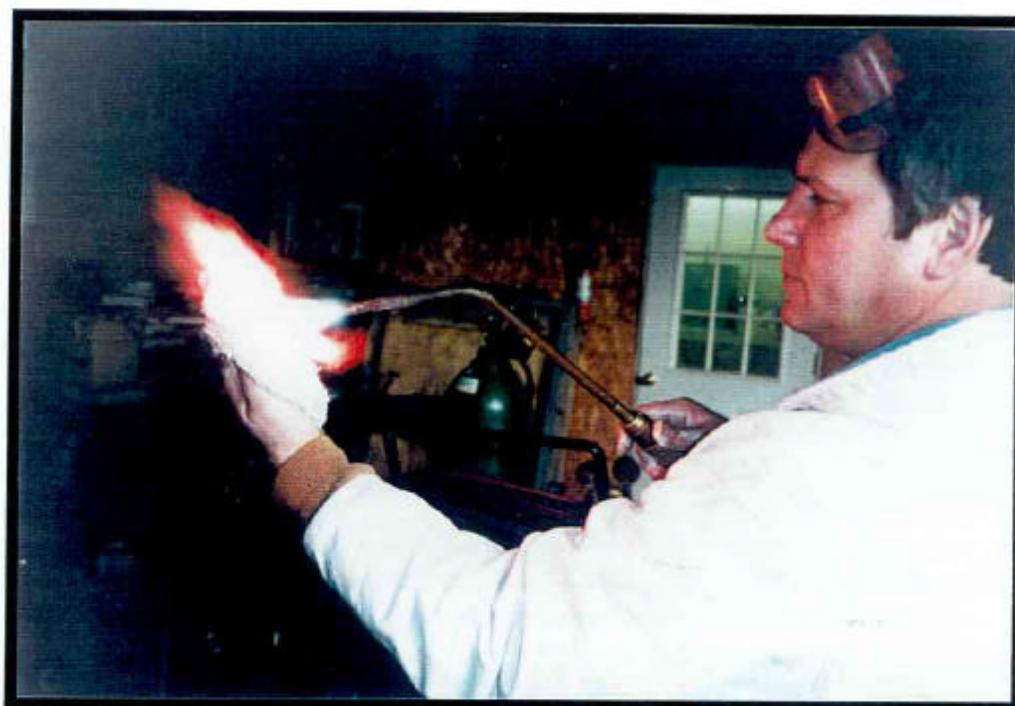
Photo shows the inventor holding a 3/8" sample of FireComp in one hand and a 5500 – 6000 degree Fahrenheit oxygen/acetylene torch in the other hand.
