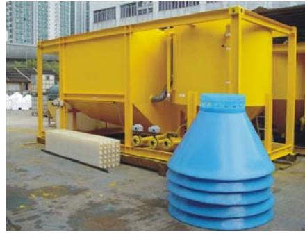
WetSep Filtration c/w 2 stages filter
