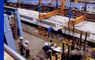
A full-size double tee beam was fabricated and tested to destruction prior to construction of Structure B.
