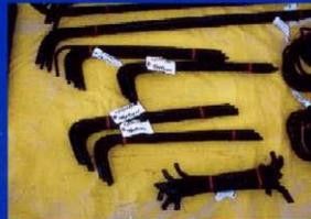
Carbon Fiber Reinforced Polymer (CFRP) is manufactured in a variety of forms including bent shapes shown here.
