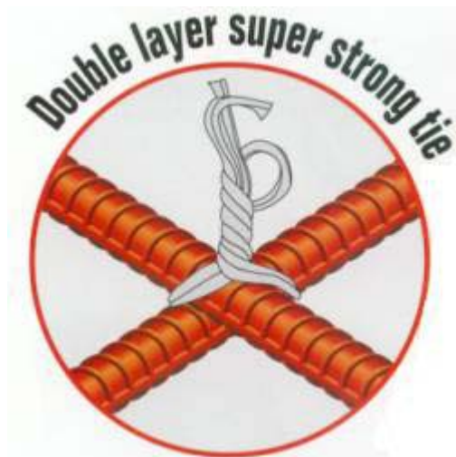
Figure 5. Schematic of joint tied with U-Tier
