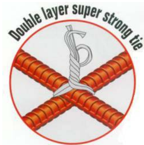
Figure 5. Schematic of joint tied with U-Tier
