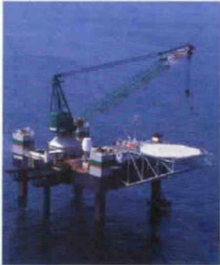
1. The IB909 jack-up barge returned to Massachusetts Bay to install a caisson and a ventilation pipe in order to bring air into the effluent outfall tunnel.
